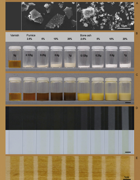
Fig. 3 Reconstructions of historical recipes. A) Scanning electron microscope images (SEM-SE) of the pumice stone (glass shards, left) and bone ash (calcium phosphate, right). B,C) Different amounts of the ground solid were added to the varnish. D) 50 µm thick films on glass, and E) varnish films on wood.
